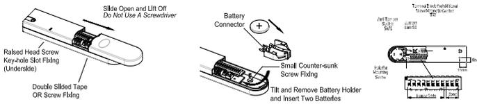
Open the sensor, take out the battery connector, and place the battery! Check the house code; same as PIR and Remote Dip 1-8 from 1-12. Select the Zone you want: setting Dip 9-11 according the overview below. Mark the Zone number on the magnet.
