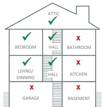
Caution: Do not install smoke alarms in areas where humidity is high or where false alarms may occur due to, for example, cooking fumes or exhaust fumes. Choose for **heat alarms** instead of smoke alarms in bathrooms, kitchens and garages. These alarms react to temperature rises and not to smoke. Visit [www.elro.eu](http://www.elro.eu) for the range of heat alarms.
