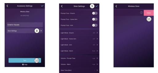
• Testing from the app is very easy, just tap test (10) in the "Accessory settings" menu of the "Exterior facade" box.
