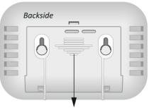
Slide down to open battery compartment
