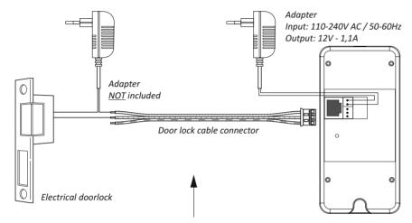
For a electrical door lock, use the upper and middle wires For a magnetic door lock, use the middle and lower wires
