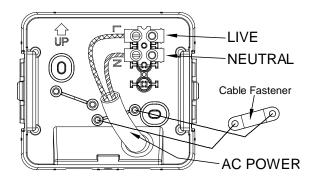
(6) Refit the Spotlight onto the wall box and secure with the two clips. Refit the wall box screw at the base of the unit (if fitted).
