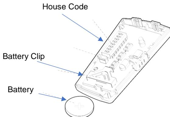
Insert the 3V (CR2032) battery. Check the house code of your system and put this also into the remote (same as in the door/window magnet and the PIR). Before you open a door/window magnet or a PIR change the Disarm ready modus of the Alarm Panel to Installation modus:
