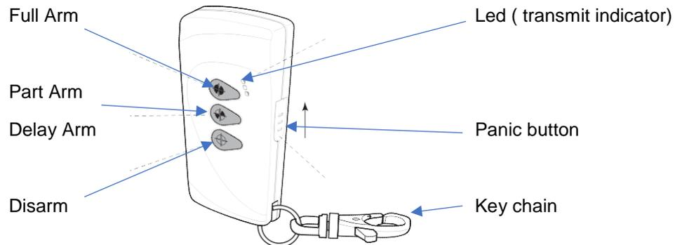
The Remote Control incorporates a Personal Attack Switch (Panic). Activating the Panic Alarm will immediately initiate a Full Alarm condition whether the system is Armed or Disarmed, (unless the system is in Service, Test or Program mode).
